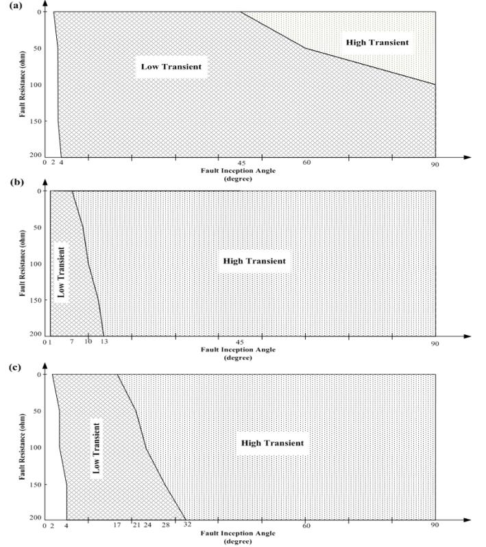
Figure 6. Operation characteristic of the (a): Relay<sub>Choghadak</sub>, (b): Relay<sub>Pars</sub>, (c): Relay<sub>Kangan</sub>, for internal LG faults at 0.5km from Pars substation
