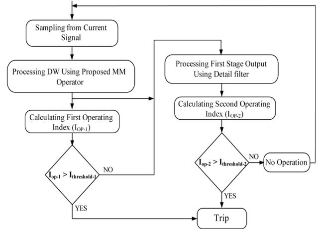
Figure 2. The flowchart of the proposed protection algorithm.
