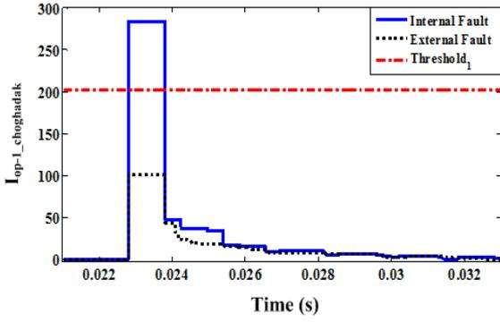
Figure 4.  $I_{op-1\_choghadak}$  for remote internal and external LG fault at 0.5 km from Pars at  $V_{90}$  and  $R_{00}$ .
