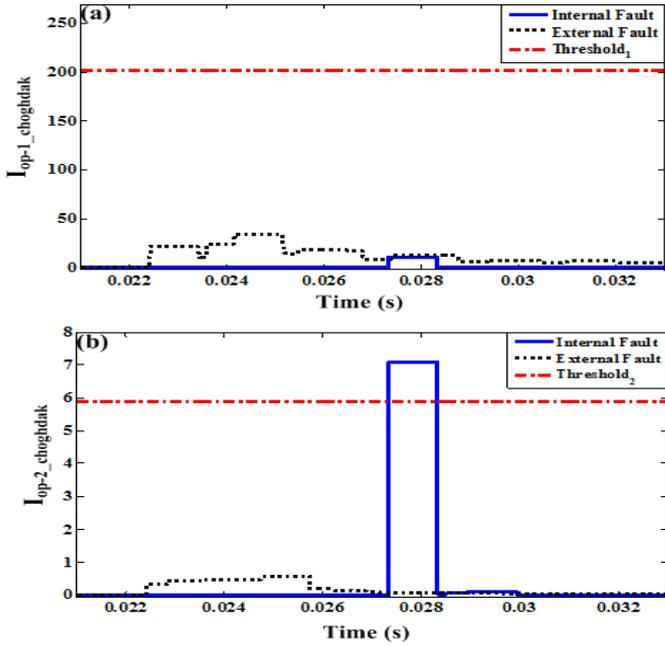
Figure 8. (a):  $I_{op-1\_choghadak}$  (b):  $I_{op-2\_choghadak}$ , for the LG close-in fault at  $V_{01}$  and  $R_{200}$  and the strongest LG close-out fault at 0.5 km from Choghadak substation
