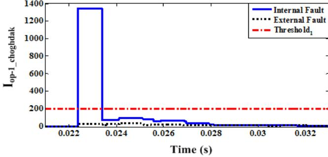
Figure 7.  $I_{op-1\_choghadak}$  for close-in and close-out LG fault at 0.5 km from Pars at  $V_{90}$  and  $R_{00}$
