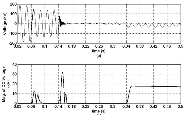
Fig. 12 Instantaneous voltage and its DC component measured by relay  $R_1$  for the 100 km-length double-circuit line
