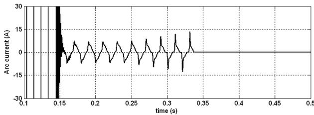
Fig. 11 Arc current at the fault branch for the 100 km-length double-circuit line
