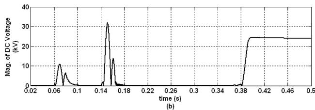
Fig. 8 Instantaneous voltage and its DC component measured by relay  $R_1$  for the 200 km-length single-circuit line
