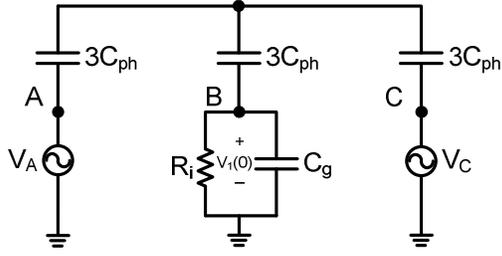
Fig. 2 Model of system shown in Fig. 1 used for obtaining  $V_B$
