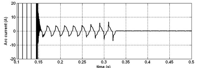
Fig. 9 Arc current at the fault branch for the 50 km-length single-circuit line
