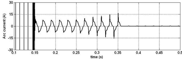
Fig. 5 Arc current at the fault branch for the 100 km-length single-circuit line
