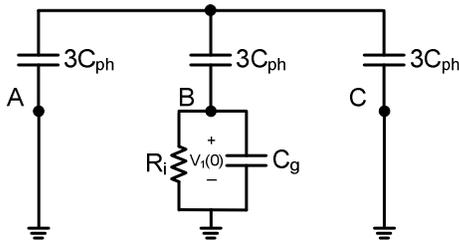
Fig. 3 Circuit used to obtain phase B voltage in the presence of initial voltage created after fault elimination
