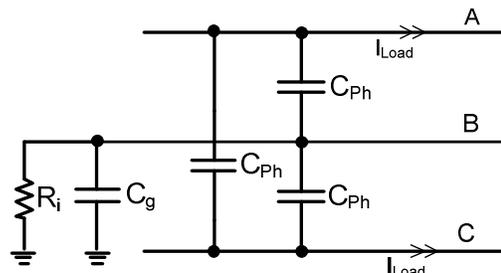
Fig. 1 A three-phase transmission line with open phase B
