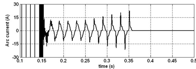
Fig. 7 Arc current at the fault branch for the 200 km-length single-circuit line
