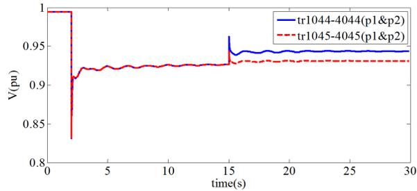
Figure 4: voltage of bus 1043 due to change of two reactive agents
