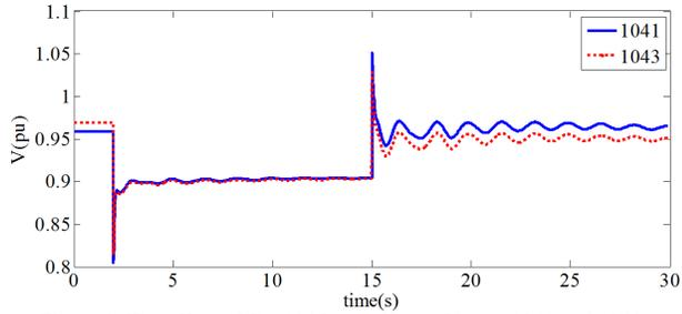
Figure 3: The effect of Cap1045 on voltage of buses 1041 and 1043.
