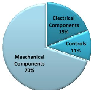
Fig. 1. Breaker failure types by major components.
