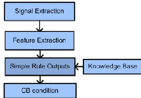
Fig. 2. Solution Architecture for CB monitoring by inspecting mechanical components
