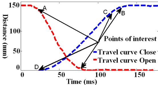
Fig. 4. Typical contact travel curves for (a) open and (b) close operation.
