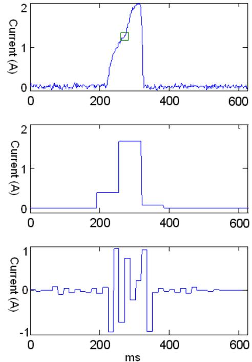
Fig. 7. Decomposition of coil current using DWT
