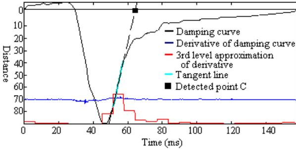
Fig. 6. Extracting the tangent line
