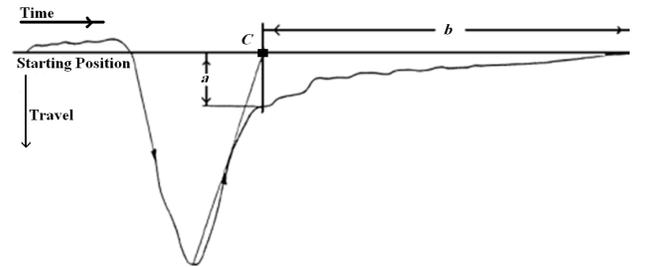
Fig. 5. CB damping curve courtesy of [11].
