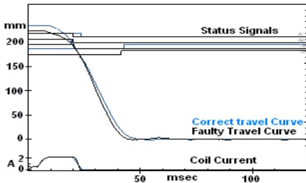
Fig. 8. A sample of a faulty travel curve signal in comparison to a correct signature [12].
